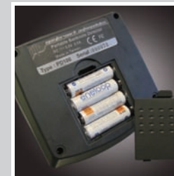
4 AA batteries, can process banknotes anywhere.
